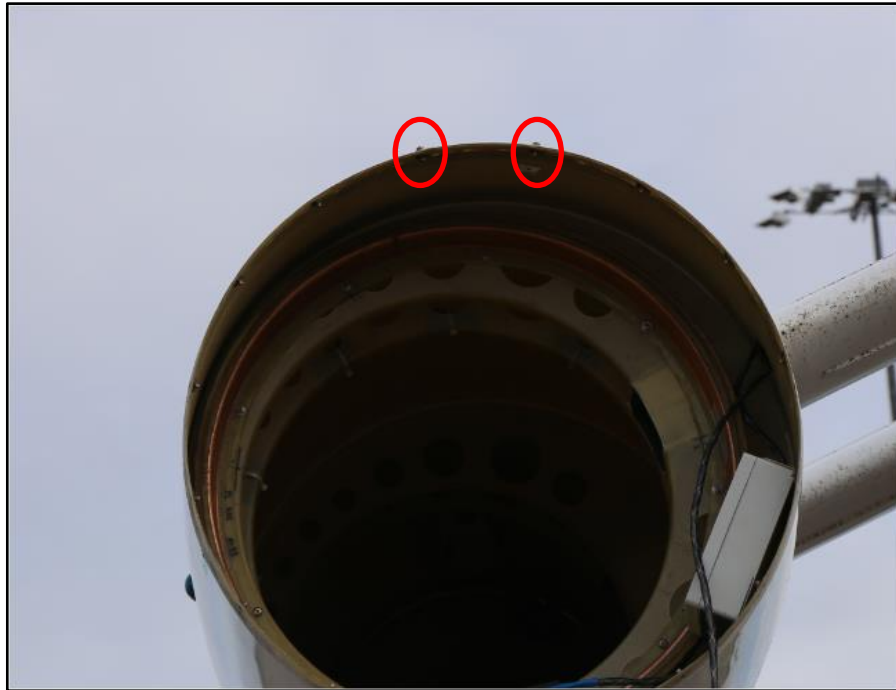
Photo No. 2: Two top screws installed on EM Pod.
