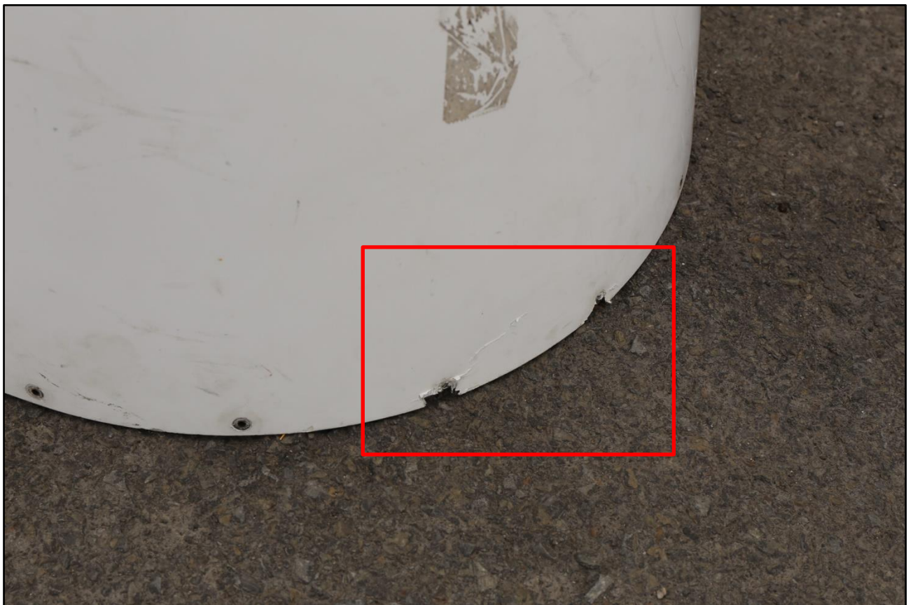
Photo No. 1: Nose cone with two retaining screw holes torn through.
