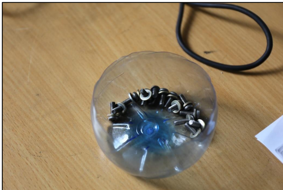
Photo No. 3: Missing nose cone retaining screws as located at the Operator's premises at EIWT.
